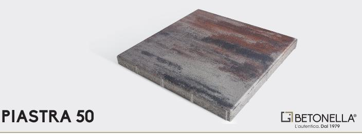
Piastra 50 is a slab particularly suitable for pedestrian areas, where a concrete screed has already been laid and where, because of the limited thickness, it is not possible to lay Betonelle (6 cm Solid concrete + 4 cm of sand). It is made with the double layer finish surface technique and for this reason it can be matched easily to a Betonella® paving.
