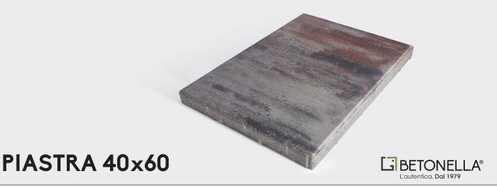
Piastra 40x60 is a slab particularly suitable for pedestrian areas, where a concrete screed has already been laid and where, because of the limited thickness, it is not possible to lay Betonelle (6 cm Solid concrete + 4 cm of sand). It is made with the double layer finish surface technique and for this reason it can be matched easily to a Betonella® paving.
